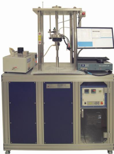
The SCC instruments of Advance Instrument (AI) are computer controlled, electromechanically operated loading devices. The loading unit can perform SSRT tests, constant load tests and cyclic fatigue tests. It is for the investigation of various forms of Stress Corrosion Cracking (SCC) under different environmental conditions.
